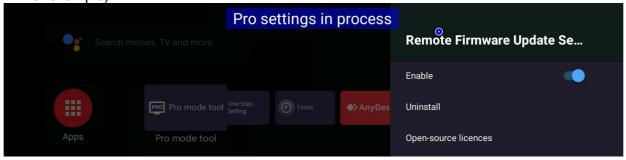
When activating "remote firmware update service" an automatic message appears to make the installation of the app, follow the installation points and reboot the device.
