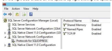
Next right click on TCP/IP and select properties. Select the IPAddresses tab. For the IPv4 address set Enabled to yes, clear the TCP Dynamic Ports field and add the port 1433
