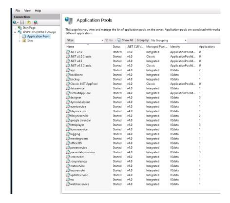
If it doesn't work try to change the password of one application manually by clicking right -> Advanced Settings. Go to Identity -> IISdata and click on the box with ...:
