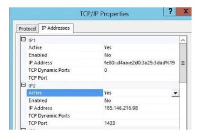
Now scroll down to the bottom, add port 1433 to the TCP Port field and click apply -> OK.
