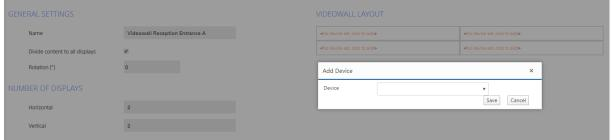
When adding all the devices, press save and go to device administration. The videowall solution will be shown as a virtual device linked with sub devices
